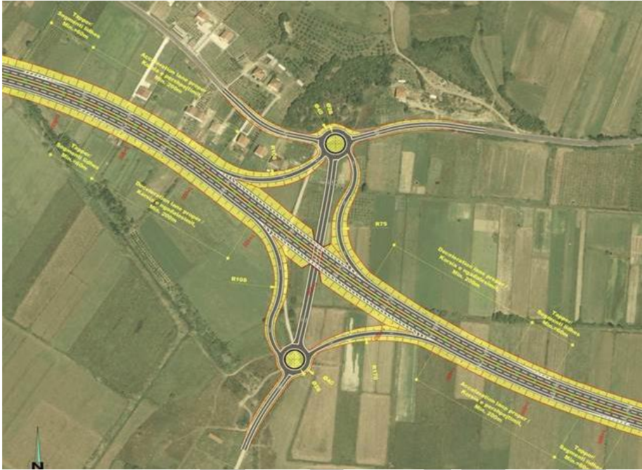
Figure 3-25 Typical layout of Type "A" (diamond) interchange
