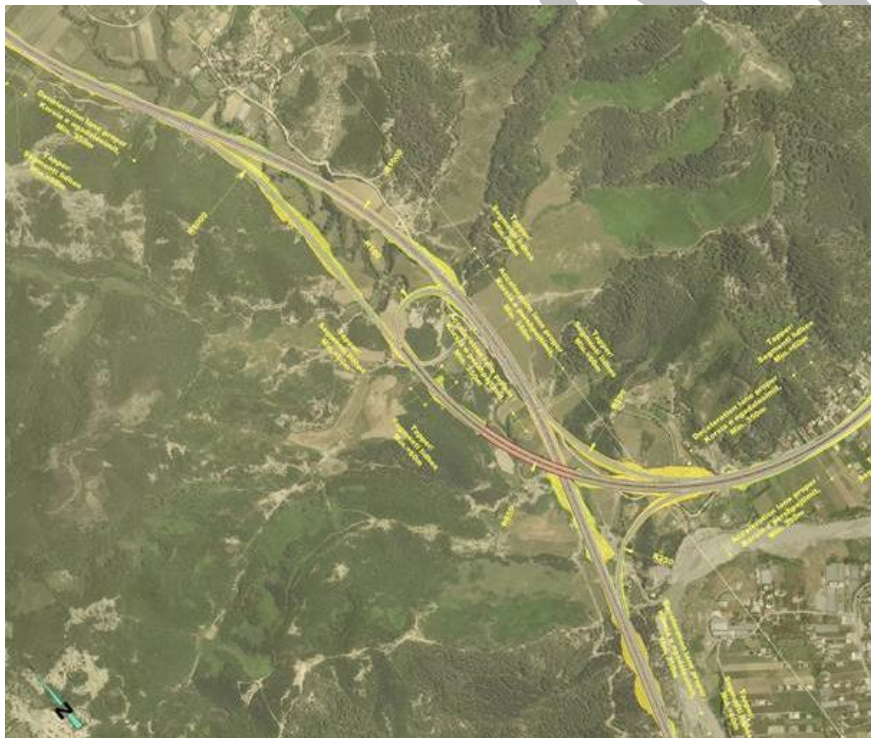
Figure 3-27 Typical layout of Type "B2" (elongated trumpet) interchange
