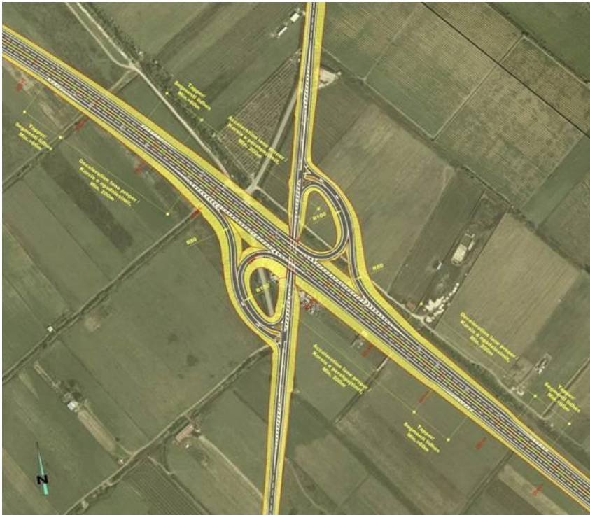
Figure 3-28 Typical layout of Type "C" (half clover leaf) interchange
