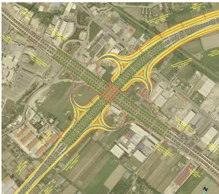
Figure 3-29 Typical layout of Type “D” (clover leaf) interchange
